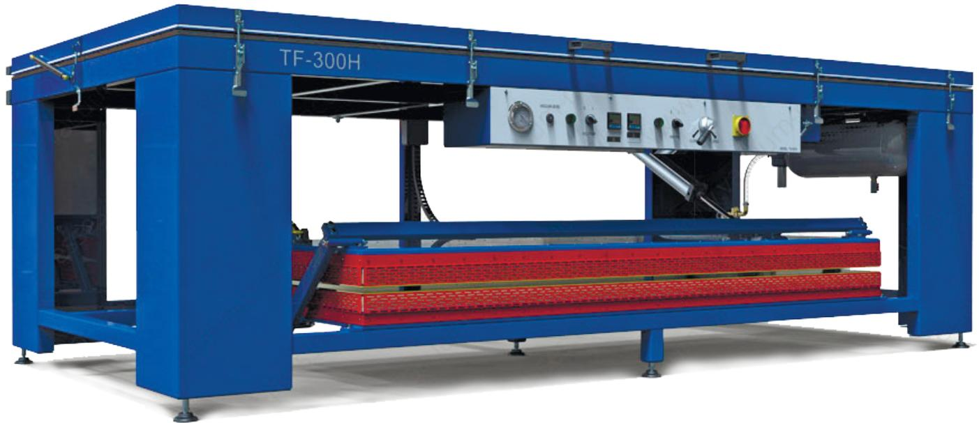
The thermoforming membrane vacuum presses TF-160H, TF-300H and TF-350H is designed special for solid surface materials (Corian, Hi Macs, Staron, Hanex, Kerrock and others) preheating and shaping, as well an acrylic material and a thermoplastic forming. Vacuum presses of TF series is combined solution which including functions of two separate machines a vacuum press and the preheating oven, greatly increases its functionality.
