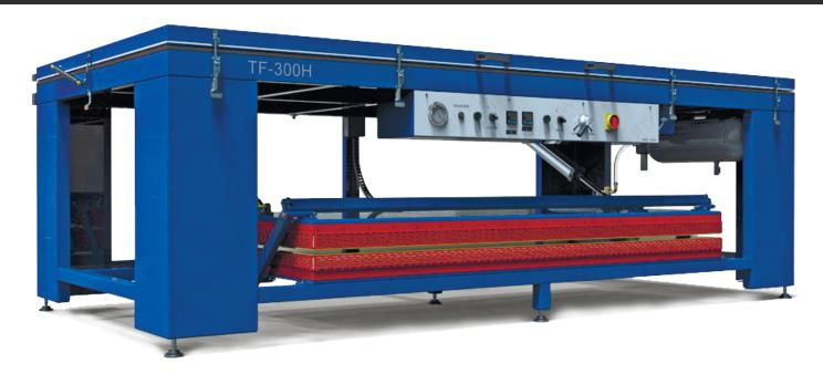
The thermoforming membrane vacuum presses TF-160H, TF-300H and TF-350H is designed special for solid surface materials (Corian, Hi Macs, Staron, Hanex, Kerrock and others) preheating and shaping, as well an acrylic material and a thermoplastic forming. Vacuum presses of TF series is combined solution which including functions of two separate machines a vacuum press and the preheating oven, greatly increases its functionality.
